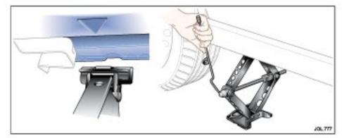
Before raising the vehicle, extend the telescopic wheel nut wrench and slacken, but do not remove the wheel nuts.
