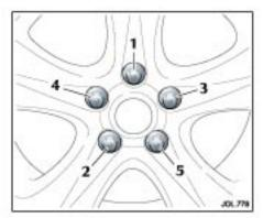
Fit the spare wheel and loosely secure with the wheel nuts.
